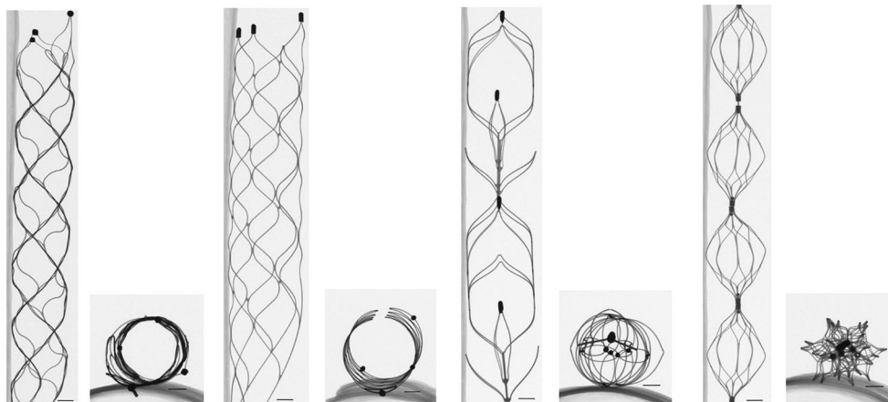
Fig. 1 Micro-CT fluoroscopy of the applied clot retrievers transversal and longitudinal; Trevo ProVue, Solitaire FR, 3D-Separator, ERIC
